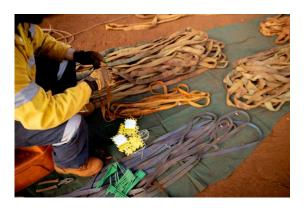
Remove the synthetic web sling from service if any of the above-mentioned issues are observed.
